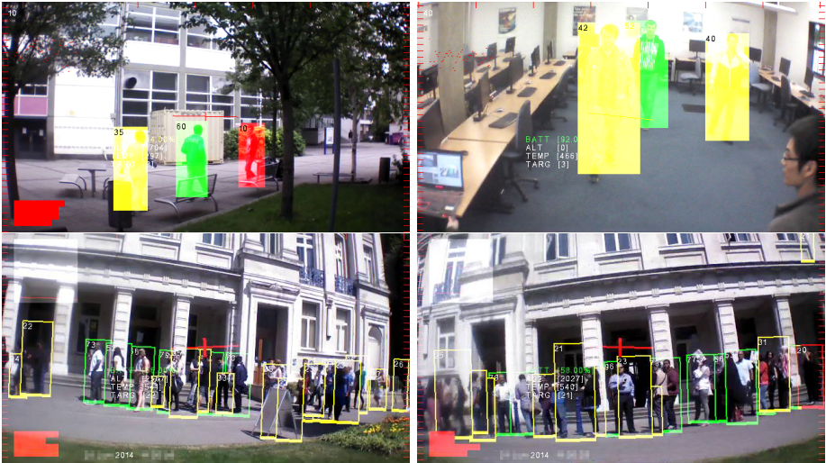
Fig. 3. Screen captures from our mobile re-identification platform’s data capture sessions; illustrating real-time person detections colour-coded by detection confidence. The top-left and top-right images illustrate typical operator views from the outdoor and indoor flights from Dataset 1; The bottom row illustrates Dataset 2.
